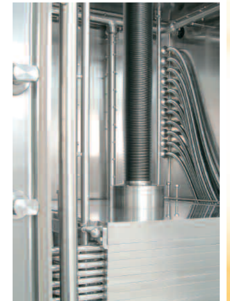
11.1.: Product chamber with shelves in lower position and stainless steel hoses for heat transfer fluid
