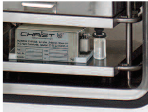
22.1.: Martin Christ weighing system specially designed for freeze drying
