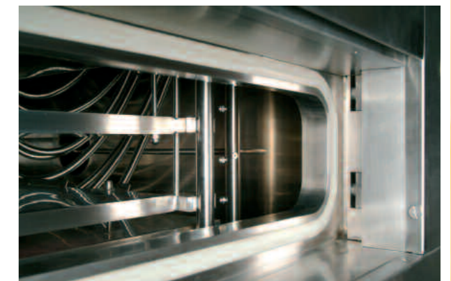
13.2.: Slot or "pizza door" on the Epsilon 2-400 DS with steam sterilization
