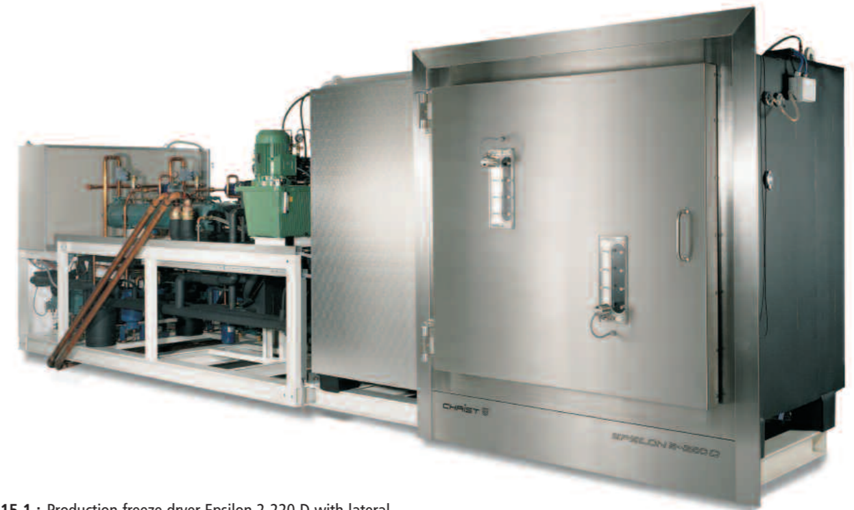
15.1.: Production freeze dryer Epsilon 2-220 D with lateral ice condenser placed next to the drying chamber (30 m 2 shelf area, 220 kg ice capacity)
