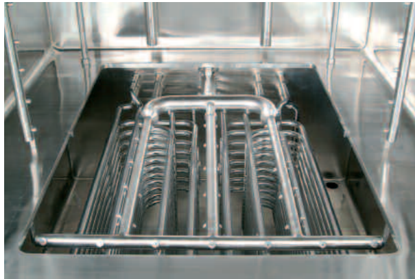
10.1.: View of ice condenser chamber (with CIP steam sterilization)
