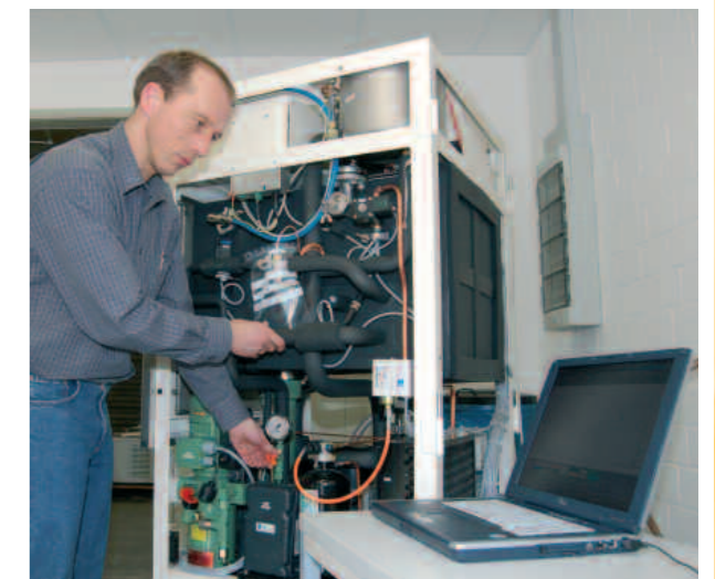
29.2.: Final inspection and test of a pilot freeze dryer
