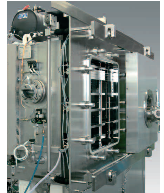
13.1.: System with sliding door
