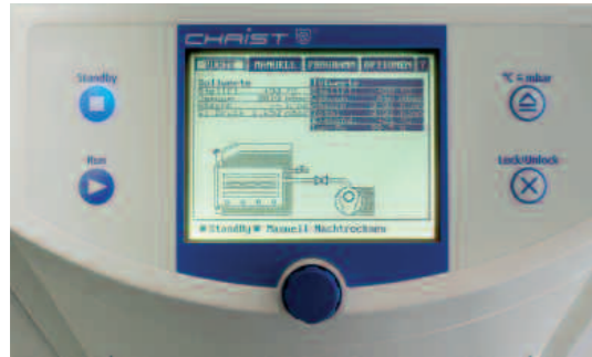
16.1.: LSC-Controller with system diagram for smaller pilot systems
