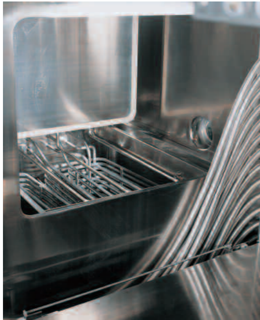
12.1.: Customized Ice condenser of an industrial unit, arranged sideways
